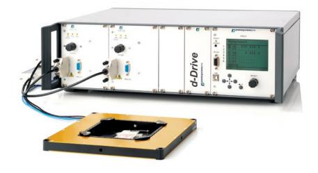
flexure system create a completely play free motion. Overshooting (oscillation) is actively minimized by controllable setting and resetting forces (generated by two different actuating systems). Even under full load pre-selected positions can be reached in milliseconds with nanometer accuracy. This is an essential characteristic especially for high-speed scanning.
